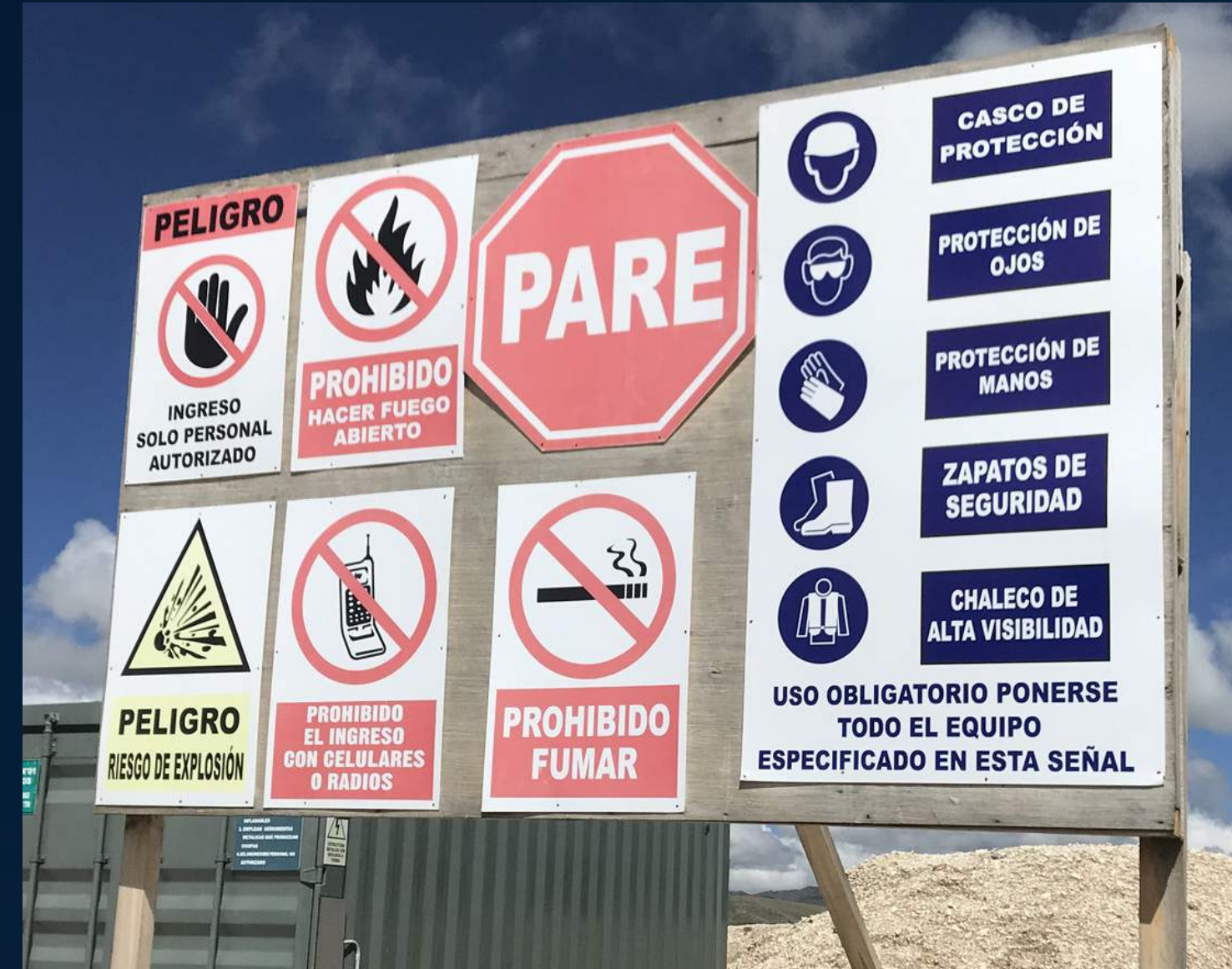
Safety poster and mandatory use of PPE in the quarry powder keg.
